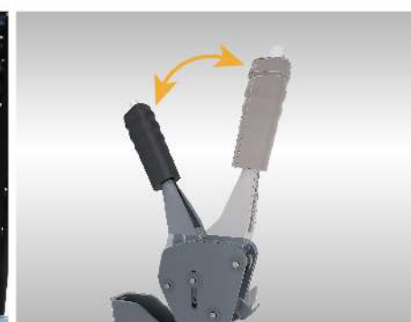
Ratchet type hand brake
