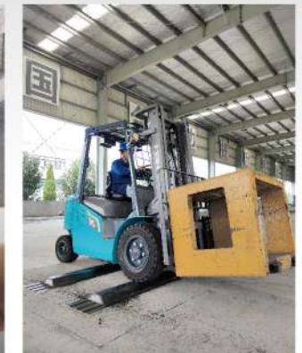
The truck passed simulation experiment of bumpy road.
