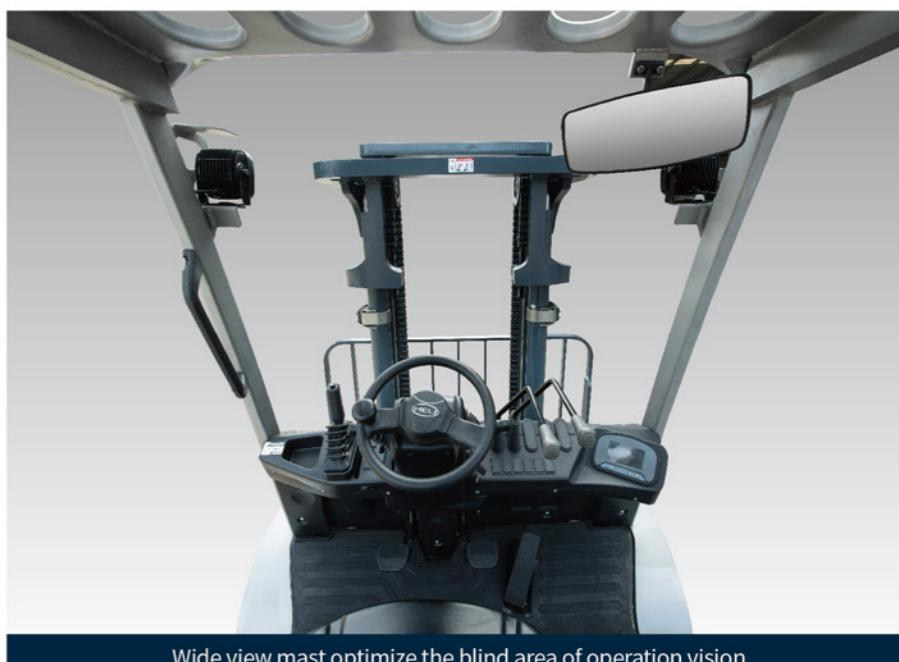
Wide view mast optimize the blind area of operation vision and it is comfortable and safe for operation;
