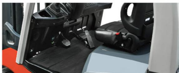
When the tilt cylinder sinks down in layout, the upper space of the bottom plate increases and the leg space is enlarged;
