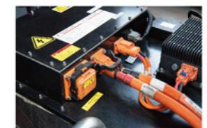
**System level voltage safety protection:** The truck features integrated / shortest design of voltage connection and multiple insulation monitoring protection;
