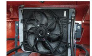
High efficiency liquid cooling and heat dissipation system is equipped as standard, which can meet the requirements of automobile S1 continuous working system;
