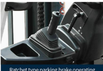
Ratchet type parking brake operating handle offers more labor-saving operation;
